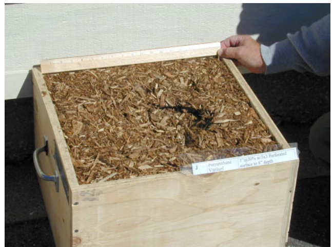
Figure 8—Polyurethane stabilized specimen after three impact events.
