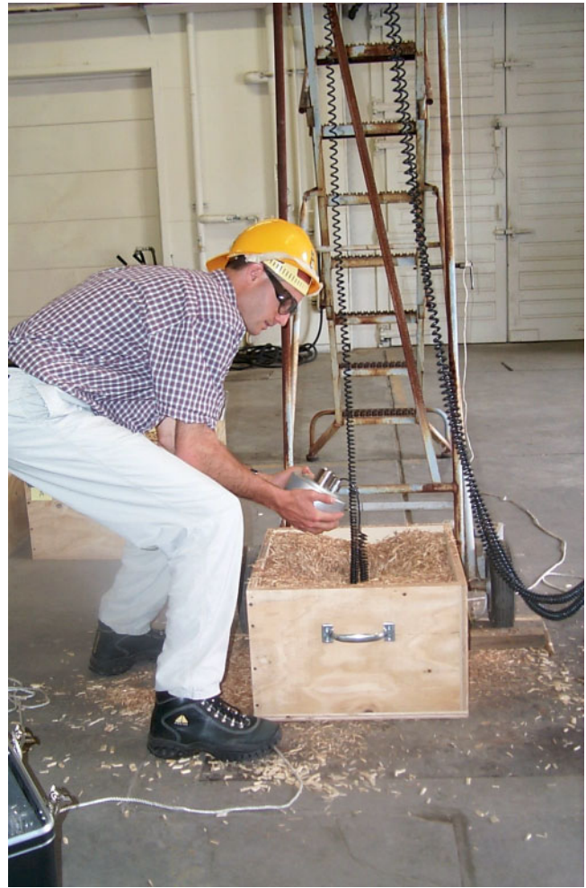
Figure 2—Impact head caught on rebound from EWF surface.
