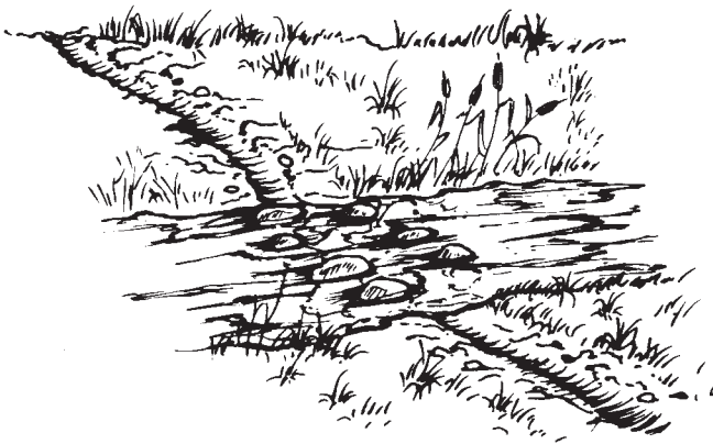
Flat stones work as effective materials for creating paved stream crossings.
