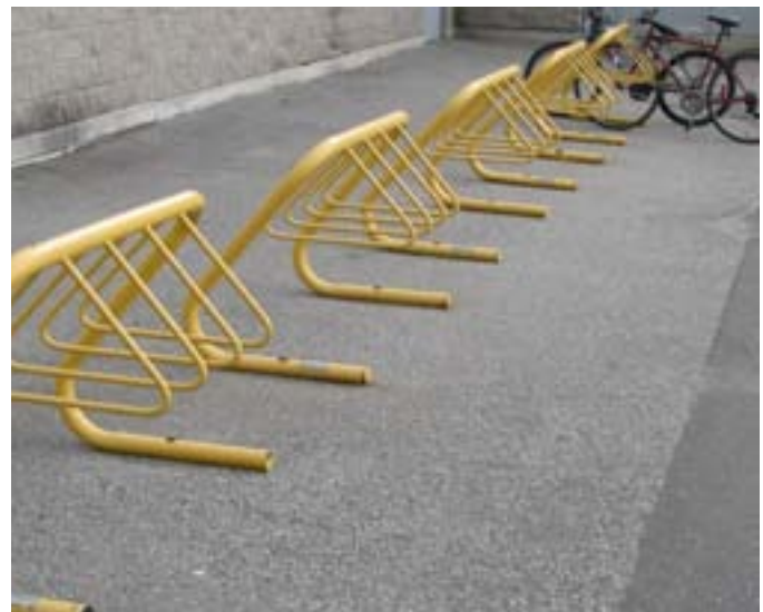
These racks park multiple bicycles and allow cyclists to lock the bicycle frame and at least one wheel to the rack.
