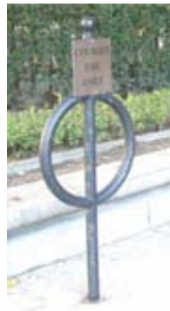
Good bicycle rack design provides 2 or more contact points between the bicycle and rack. A tapping rail close to the ground would improve the rack on the right by making it more easily detectable for blind or visually impaired people.
